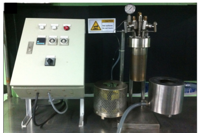
Figure 3: Innovative sanitation technology (top to bottom): Solar septic tank; hydrothermal carbonization of fecal sludge
