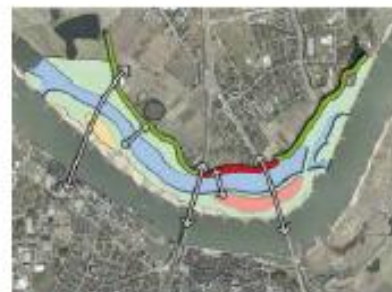
Figure 2: The ‘Room for the River’ plan at Nijmegen. The green line indicates the current line of the protective dike. The red line shows the position of the proposed relocated portion of dike. In the bottom image, the new river channel is shown in blue and the new island in yellow/green. The white arrows represent the bridge connections planned for the island. Source: Nijssen and Schouten, 2012 13 .
